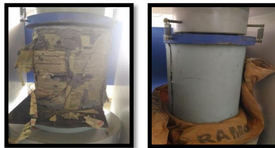
Fig.2 RC column showing crack patterns and CFRT Column showing buckling effect on axial load test under compressive testing machine.
