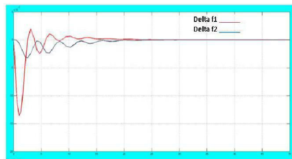
Fig.6 : \Delta f_1 and \Delta f_2 with AGC-ACE loop
