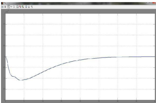
Fig.11: \Delta P_{tie} with PID controller tuned by Z-N method
