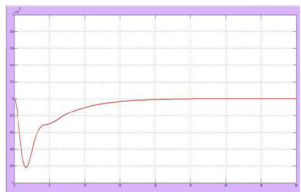
Fig.12: \Delta P_{tie} with PID controller tuned by Simplex method
